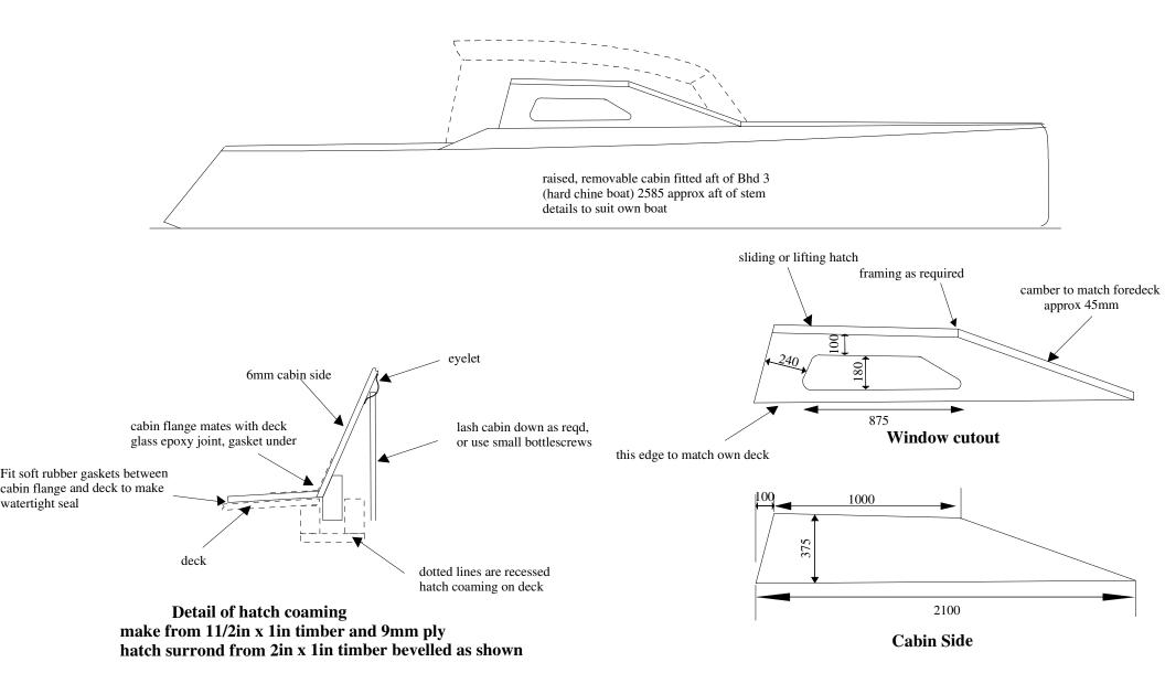
make from 6mm ply with timber framing or glass tape joints as reqd cabin width to suit own boat, ensure daggerboard can still be used Cabin sides angle in approx 15deg
